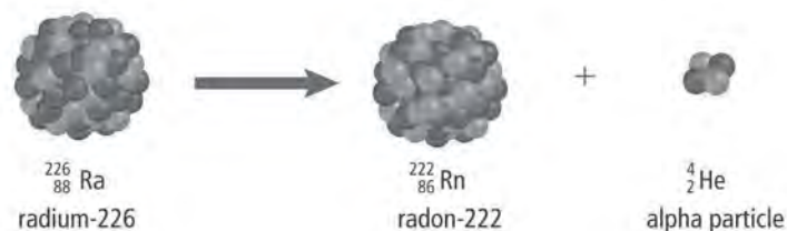
FIGURE 7.1 A radium-226 nucleus undergoes alpha decay to form a different element, radon-222, and an alpha particle.
