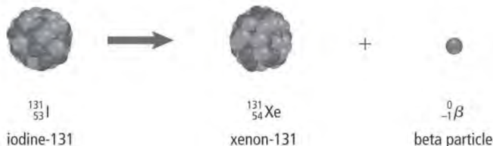
FIGURE 7.2 An iodine-131 nucleus undergoes beta decay to form a different element, xenon-131, and a beta particle.
